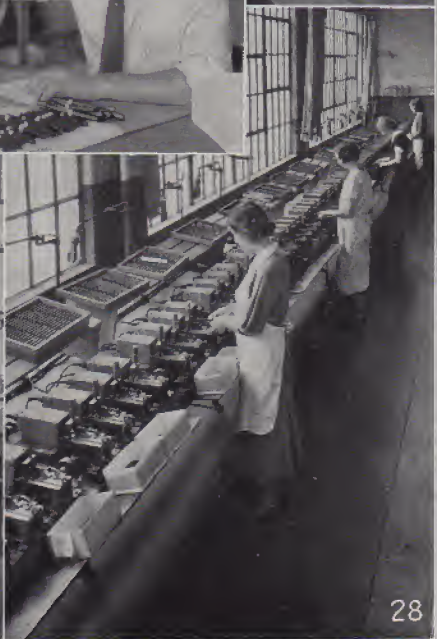
27—Fitting nibs and feeds. 28—"Heater boxes" for molding feeds to nibs. 29—General view of assembling department. 30—Final inspection of the completed pen. 31—Smoothing pen point during final inspection.
